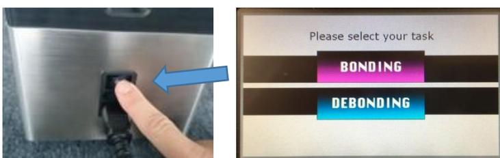
**Step 5: Chose between the programs BONDING or DEBONDING.** After clicking on BONDING you can see the screen in the middle. Please press START to get to the BONDING screen on the right.
