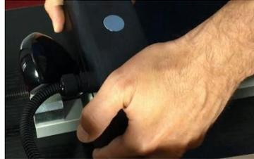
Put the club into an extraction tool and chose DEBONDING on the touch screen. If the hosel is long enough, you can use the standard **gap coil (1)** for debonding. Take it out from the generator and press it over the hosel. The debonding process starts if you press down the contact pin in the coil gap with the club head. Heat up the hosel **until you can see a little smoke plume**.
