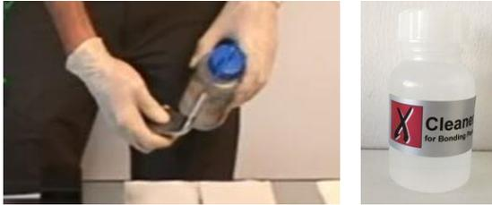
**Step 2: Treat both partners with speedXbond primer and make sure that both partners (especially the blind hole in the head) are dry before applying the adhesive (wipe on, wipe off)**
