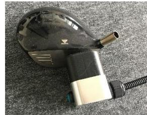
If the heat was enough to destroy the bonding **the head will be separated from the shaft by an axial force caused** by turning the pull-off spindle of the extracting tool.
