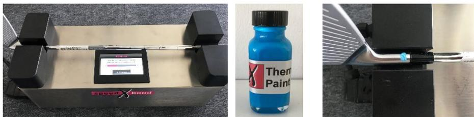
**Step 7: Start the bonding process** by pushing down the contact pin with the hosel. The pink bar begins to grow. Remove the club immediately, when the blue color of the Thermo Paint on the hosel disappears.
